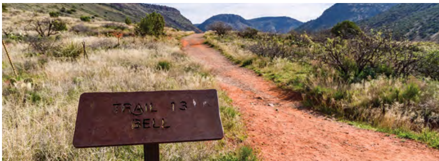
Figure 4-080—Always identify the trail as it leaves a trailhead. Provide a clearly visible entrance to the trail and define the start of the trail.
