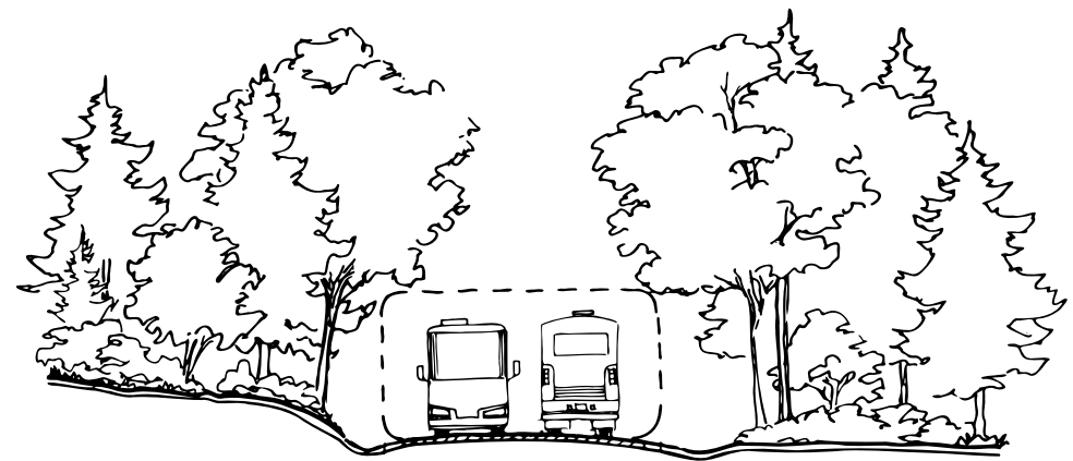
Figure 3–029—Generally, recreation site roads have minimal width and clearing, and trees and vegetation come close to the side of the road to retain the natural character of the site.
