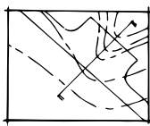
Figure 3-073—Explore and evaluate alternative design approaches early in the project development process to find a grading solution that reduces necessary cut and fill or the need to borrow from another site. These illustrations are adapted from the “Low-Volume Roads Engineering Best Management Practices Field Guide.”
