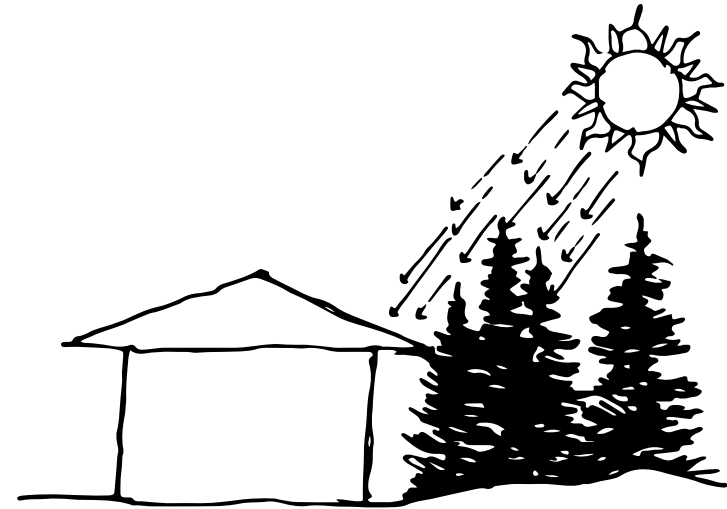
Figure 4-020—Use existing vegetation or pavilions to provide shade from the afternoon sun. This illustration is adapted from “The Built Environment Image Guide for the National Forests and Grasslands.”
