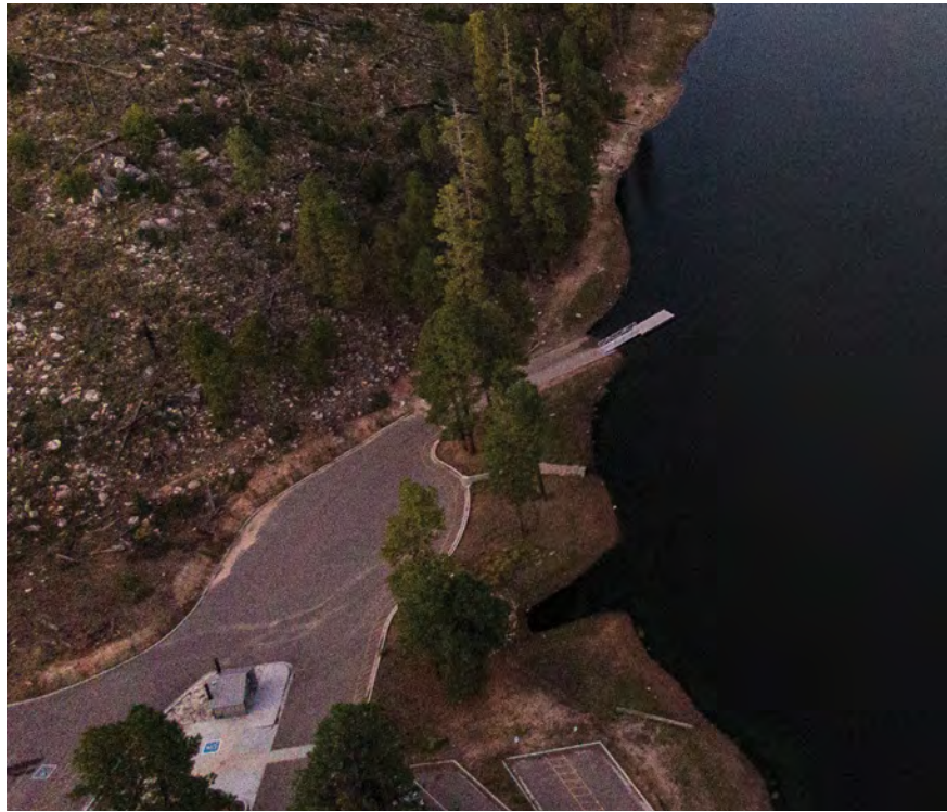
Figure 4-089—A higher development site such as this one will often have paved parking for larger vehicles and trailers, a courtesy dock, a restroom, and well-thought-out circulation.
