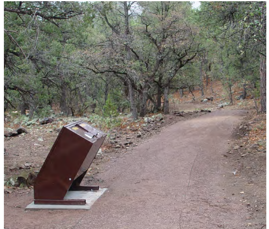
Figure 3–110—In settings where animals cause issues with waste, specify use of animal-proof garbage containers to prevent the spread of waste materials and litter and to protect wildlife.
