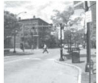
Curb extensions reduce pedestrian crossing distances and improve visibility for pedestrians and motorists alike.
