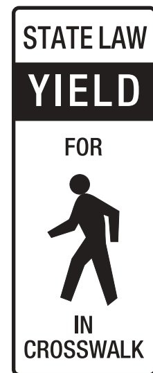
Figure 3-37. In-Street Pedestrian Crossing Sign, Layout
