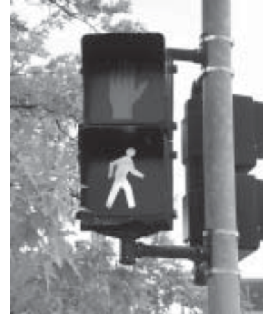
All new pedestrian signal indications shall be displayed within a rectangular background and consist of symbolized messages.
