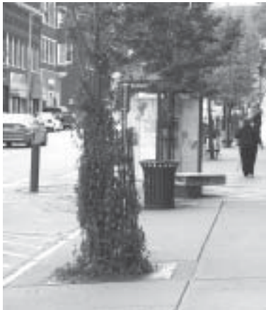
The Buffer Zone “buffers” pedestrians from the roadway and provides a place for trees, signal poles, signs, street lights, bicycle parking, and snow storage.
