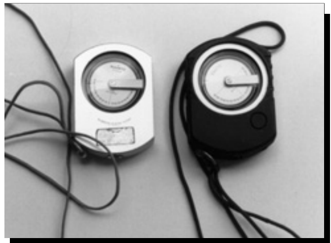
Figure 74—Use a clinometer to set grades for preliminary trail layout.
