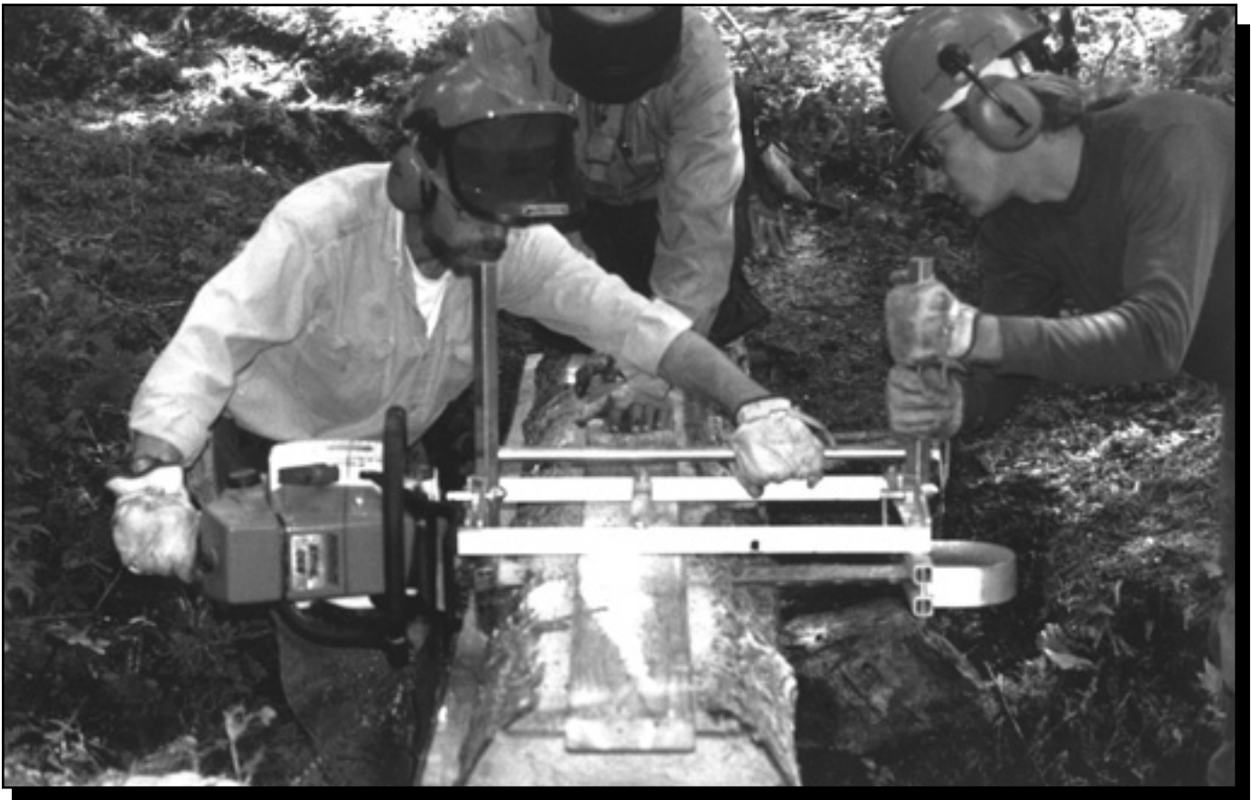
Figure 97—An Alaskan sawmill works great for creating planks from native logs. The mill requires a powerful chain saw (at least 3.8 cubic inches of displacement, more is better) and a special ripping chain.
