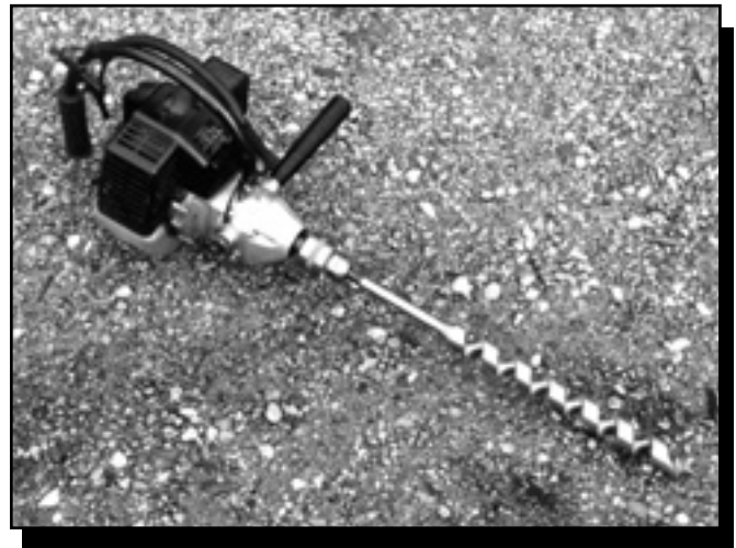
Figure 85—Gasoline-powered drills are great for backcountry work if regulations allow their use.
