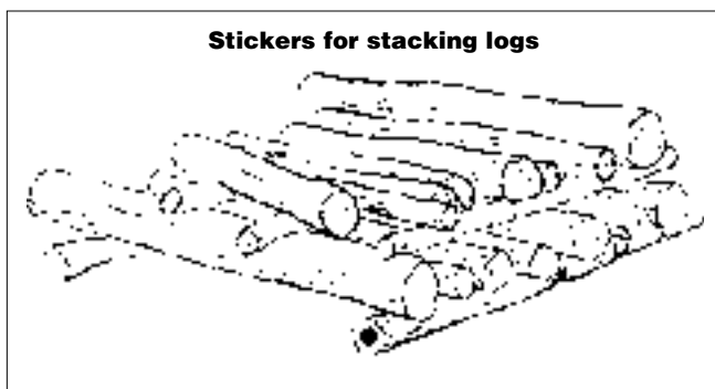
Figure 91—Stickers placed between layers of logs help the logs dry faster and reduce decay.
