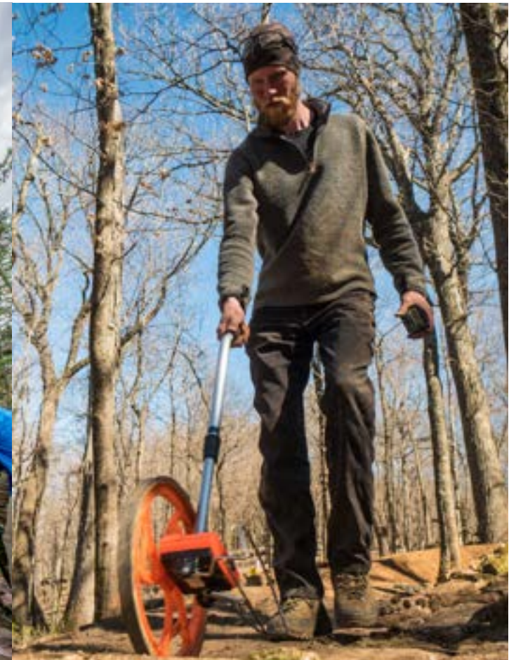
Measuring production quantities for invoice billing. Photo by Eli Glesmann/Rock Solid
