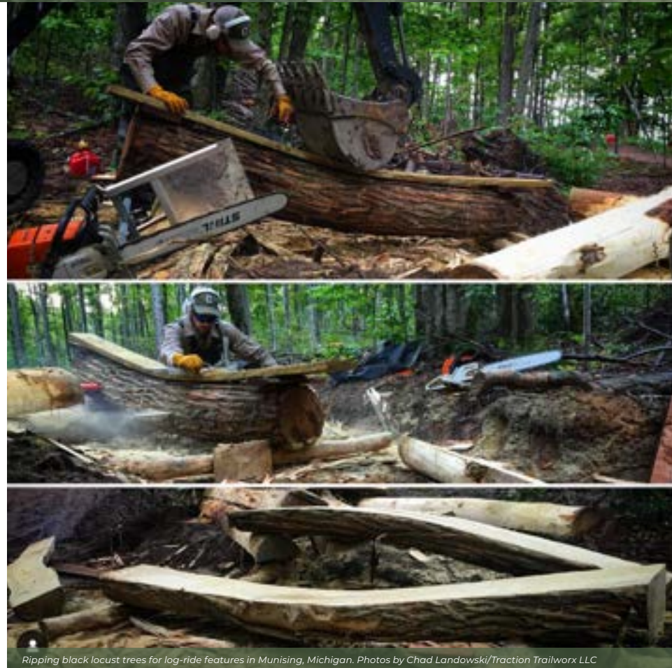
Portable chainsaw mill for planing logs in the field. Photos by Chad Landowski/Traction Trailworx
