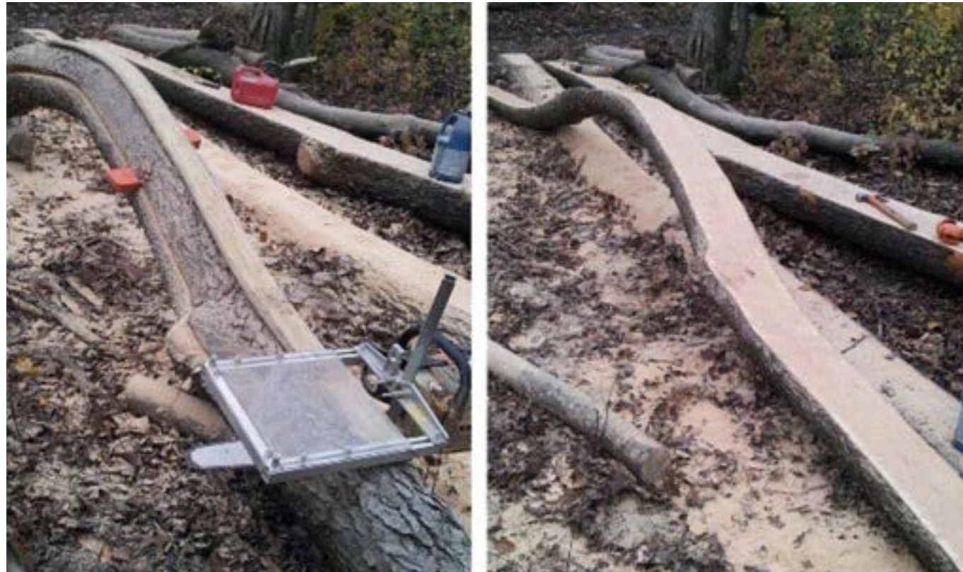
Portable chainsaw mill for planing logs in the field. Photos by Chad Landowski/Traction Trailworx
