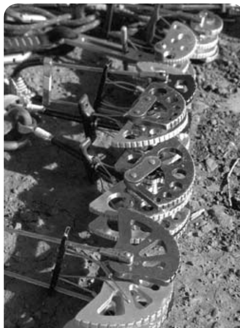
Examples of camming devices used by climbers for protection in large cracks. These spring-loaded devices are removed by manually retracting the spring and leave no trace on the rock. Photo: K. Pyke
