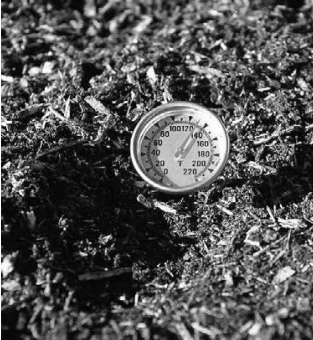
Figure 1. Probe to measure compost temperature (Fahrenheit).
