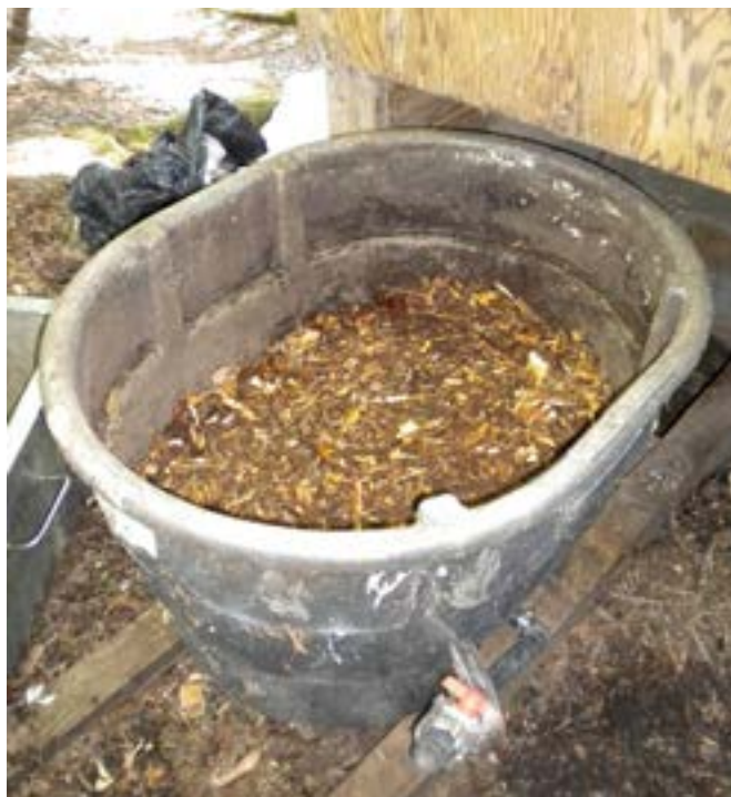
Strain plate primed with bark mulch
